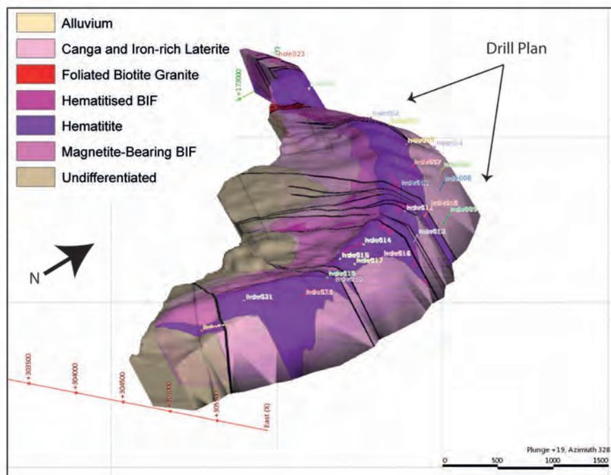
Figure 6 : Badondo 3D geology and structural model of recommended drill targets.
