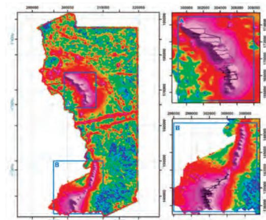
Figure 2 : Analytical signal magnetic data and GPS track logs over the Badondo (A) and Belinga North (B) anomalies
