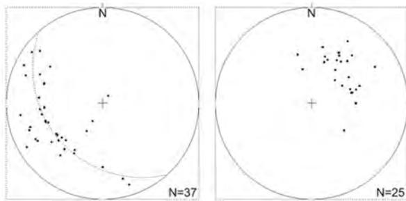
Figure 4 : Equal area stereoplots for S1 and S2 foliations (left) and L2/1 lineations at Badondo Hill
