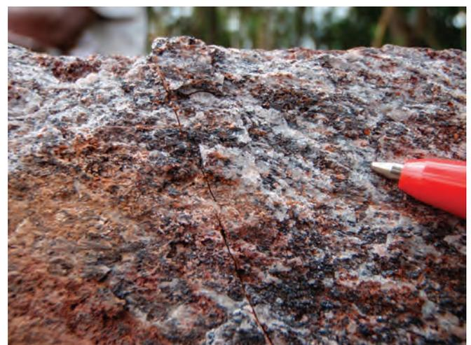
Figure 1: Close-up of a coarse-grained magnetite-bearing partly oxidised quartzite
