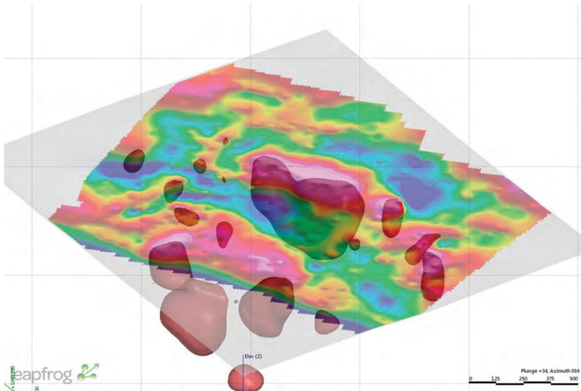
Figure 3: Results of the 3D inversion compared to the map of residual complex gravity anomaly
