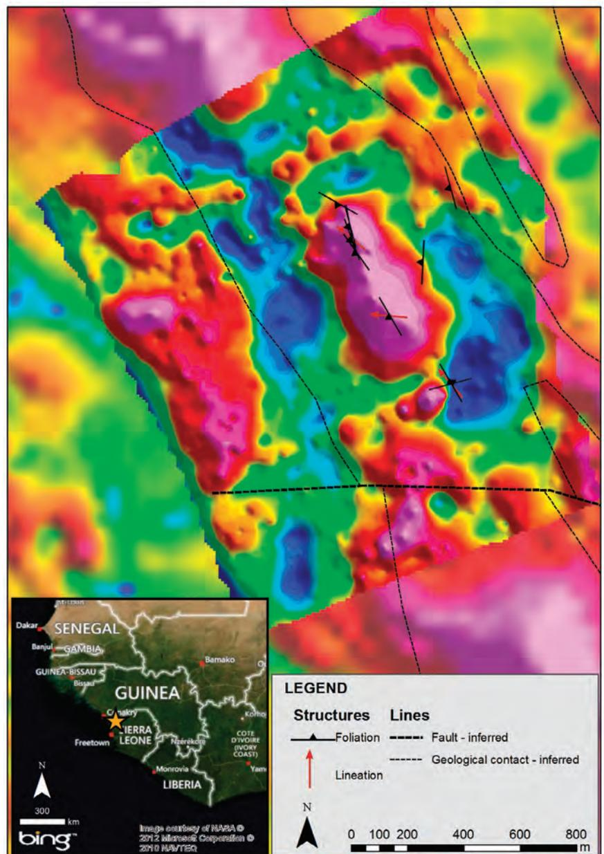
Figure 2. Residual complex  $2.67 \text{ g/cm}^3$  terrain-corrected gravity anomaly over the airborne magnetic survey (analytical signal). Structural measurements are displayed and show west-dipping foliations and NNW-trending lineations
